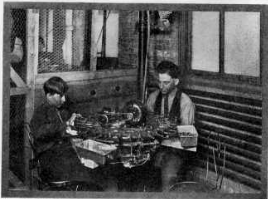
Fig. 3. A grid leak capping machine, the only device of the sort to be found in this country, for it was developed by the Daven Company.
